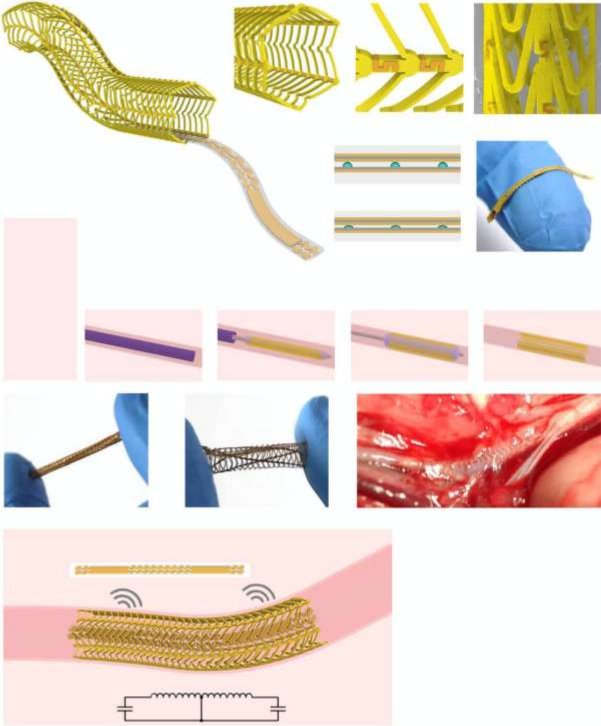
Overview of a fully implantable, wireless vascular electronic system with printed sensors for wireless monitoring of hemodynamics. (A) Illustration of the implantable electronic components. (B) Inductive stent design using conductive Au loops and nonconductive polyimide (PI) connectors to achieve a current path resembling a solenoid (left) and an scanning electron microscopy (SEM) image of the stent (right). (C) Layers of the soft pressure sensor using a printed dielectric layer (left) and photo of index finger holding a simultaneous flow and pressure sensor (right). AgNP, silver nanoparticle; PDMS, polydimethylsiloxane. (D) Illustration of minimally invasive catheter deployment and balloon expansion of the wireless vascular stent. (E) Initial and expanded state of the sensor-integrated stent system. (F) Wireless stent system implanted in the right iliac artery of living rabbit. (G) Illustration of the wireless design and sensing scheme to simultaneously monitor pressure, heart rate (HR), and flow.
